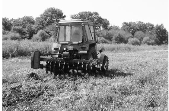
Fig9 Tractor with rotor discs is developing a firebreak.
